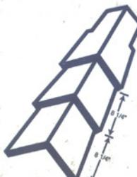
OVERLAP ALL RIDGES TO CUT OUT. FOR MAXIMUM COVERAGE MAINTAIN AN 8 1/4" EXPOSURE.
